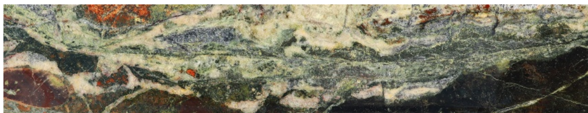
Image 15. Hole NEDD018 – 322.85m: Chalcopyrite–bornite bearing, structure-controlled quartz–calcite–chlorite vein within volcaniclastic conglomerate, returning elevated copper (1,285 ppm) and molybdenum (11.25 ppm), with minor gold and silver
