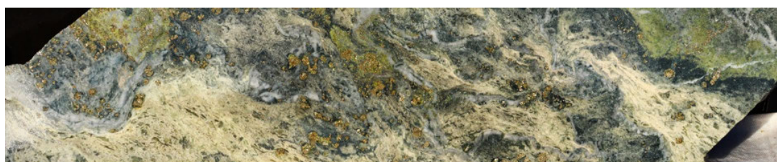
Image 18. Hole NEDD018 – 432.6m: 2–3% pyrite with chalcopyrite associated with irregular chalcidony–epidote–calcite veins within chlorite–illite–smectite altered intermediate volcanic rock, returning elevated arsenic (132.5 ppm) and molybdenum (7.55 ppm), with minor silver and copper
