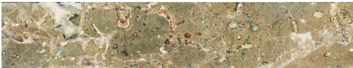
Image 20. Hole NEDD018 – 451.75m: Colloform-banded chalcidonic veins within sericite–clay altered intermediate volcanic rock, returning arsenic (10.4 ppm) and molybdenum (1.54 ppm)
