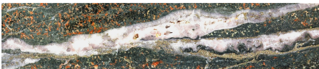
Image 9. Hole NEDD011 – 472.9m: Chalcopyrite–pyrite bearing epithermal-type quartz–calcite–K-feldspar veins with disseminated pyrite within equigranular quartz diorite, returning elevated copper (704 ppm) and molybdenum (179.5 ppm), with minor gold and silver
