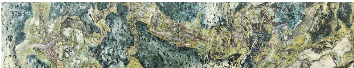
Image 19. Hole NEDD018 – 436.4m: Chalcopyrite–pyrite-bearing irregular chalcedony–epidote–calcite veins within chlorite–illite–smectite altered intermediate volcanic rock, returning elevated arsenic (55.6 ppm) and molybdenum (1.84 ppm), with minor silver and copper
