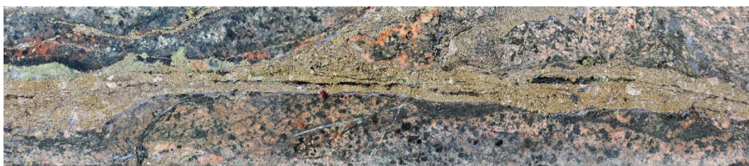
Image 8. Hole NEDD011 – 466.4m: Chalcopyrite–pyrite bearing quartz–calcite–epidote vein within equigranular quartz diorite, returning elevated copper (1,525 ppm) with minor gold, silver and molybdenum
