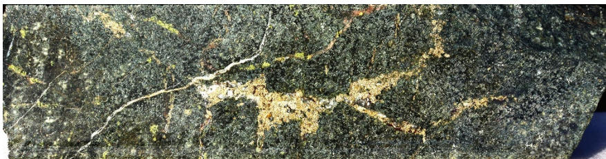
Image 13. Hole NEDD011 – 584.2m: Chalcopyrite–pyrite bearing quartz–calcite–hematite vein within equigranular quartz diorite, returning elevated copper (243 ppm) with minor gold, silver, molybdenum and zinc
