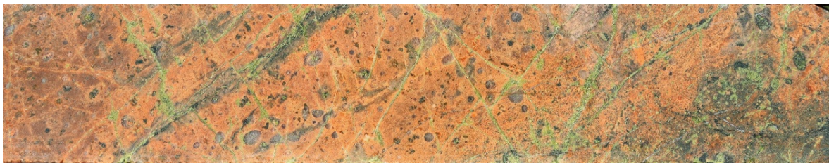
Image 12. Hole NEDD011 – 565.25m: Chalcopyrite–pyrite bearing quartz–specular hematite vein within quartz diorite, returning elevated copper (656 ppm) with minor gold, silver, molybdenum and zinc
