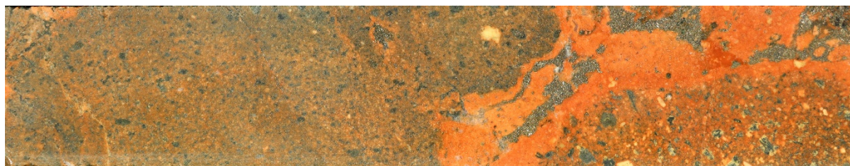
Image 2. Hole NEDD011 – 332.85m: Pyrite-chalcopyrite bearing Quartz-Monzonite-Porphyry (QMP) finger, returning elevated copper (575 ppm), molybdenum (17.9 ppm) and lead (410 ppm), with minor gold and silver
