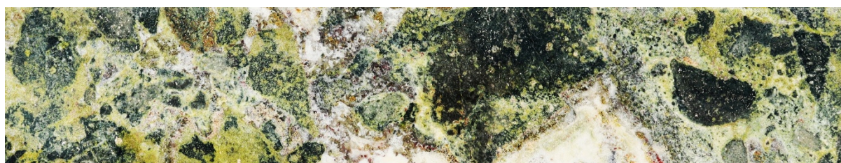
Image 16. Hole NEDD018 – 412.4m: Disseminated pyrite with colloform-banded chalcidonic vein within phyllic (QSP) altered, brecciated intermediate volcanic rock, returning copper (65.8 ppm), arsenic (40.8 ppm) with minor silver
