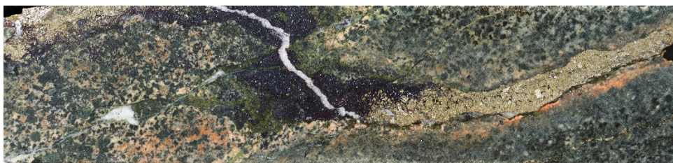
Image 7. Hole NEDD011 – 461.7m: Chalcopyrite–pyrite bearing quartz–calcite–magnetite vein within equigranular quartz diorite, returning elevated copper (611 ppm) with minor gold, silver and molybdenum
