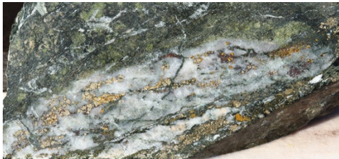
Image 10. Hole NEDD011 – 478.6m: Chalcopyrite–molybdenite bearing B-type quartz–magnetite veins within calc-alkaline quartz diorite, returning elevated copper (399 ppm) and molybdenum (118.5 ppm), with minor gold, silver, arsenic and zinc
