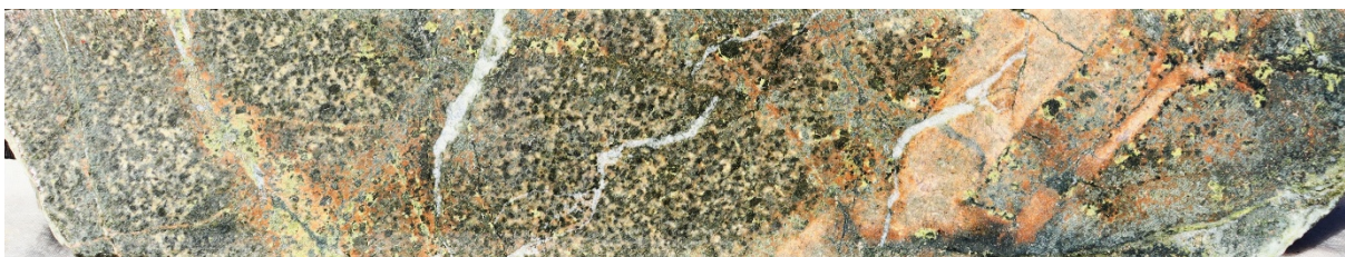
Image 14. Hole NEDD011 – 584.75m: Quartz diorite hosted felsic intrusive finger, returning elevated copper (243 ppm) and molybdenum (2.27 ppm), with minor gold, silver and zinc
