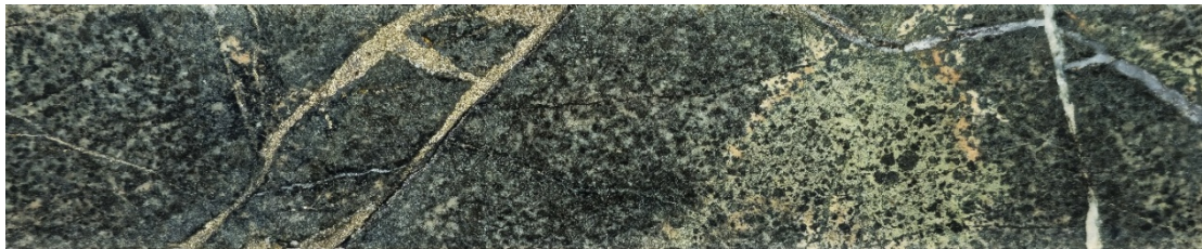
Image 6. Hole NEDD011 – 460.2m: Chalcopyrite–pyrite bearing porphyry-style quartz–magnetite and pyrite–chalcopyrite–magnetite veins, with disseminated pyrite within equigranular quartz diorite, returning elevated copper (1,150 ppm) with gold (0.307 g/t) and minor molybdenum and silver
